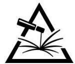
Protect the entire welding area. Compressed gas containers and other inflammable material must be moved to a minimum safe distance of 11 meters. A fire extinguisher must be readily available.
